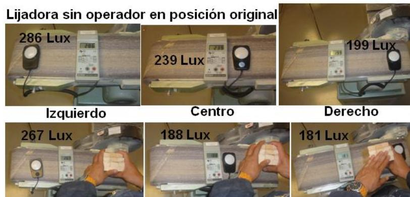
Figure 2. Lighting in Belt/Disc Sander, with operator and without
