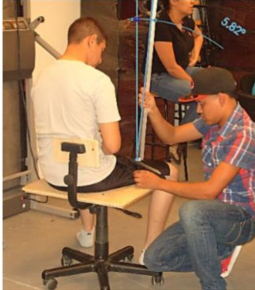
**Figure 1. Incorrect placement of anthropometer.**
