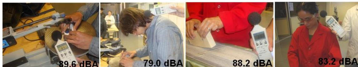
Figure 4. Some levels of noise measurements in machine and operator
