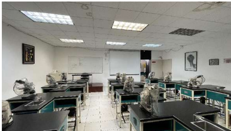
Figure 4. Layout of microscopy workstations. The prevalence of fixed-height benches and non-adjustable stools correlates with the high ROSA scores and cervical strain reported by users during prolonged visualization tasks.
