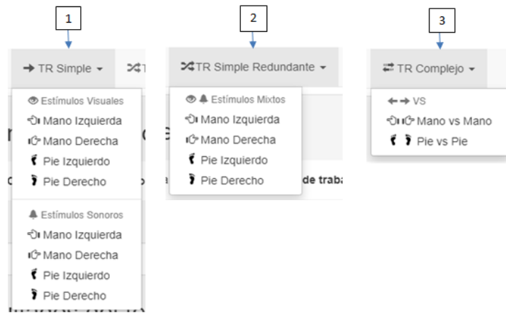
Figure 5. AMIS software menu to measure different variants of Reaction Time.
