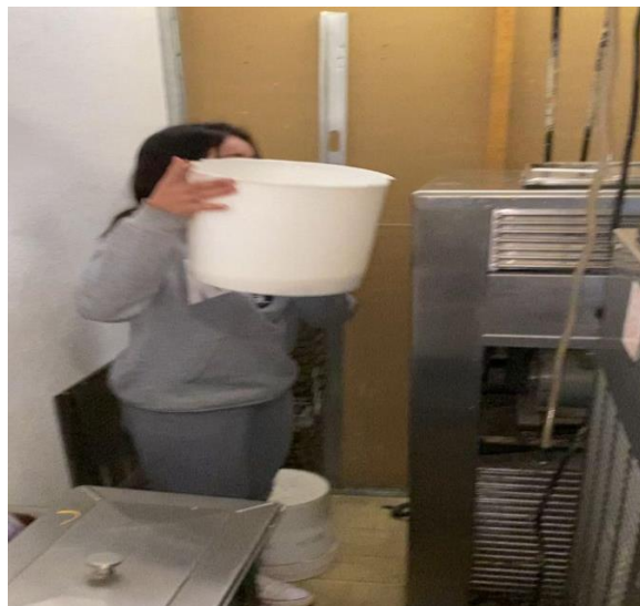
Figure 4. The initial position for filling ice cream machine or Iced Coffee machine
